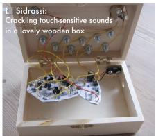
If you have circuit-bent previously, or have electronics experience and want to build something from 'scratch' then print out the "lil sidrassi" circuit and glue it onto a piece of cardboard (cereal box is ideal), and punch holes with a needle. The printout can be found here: <a href="http://www.ciat-lonbarde.net/paper/man/lilsid.gif">http://www.ciat-lonbarde.net/paper/man/lilsid.gif</a>
